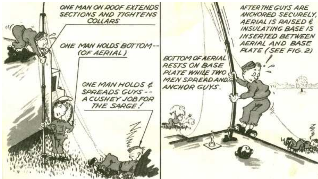
Erecting a vertical aerial on roof of a vehicle.
